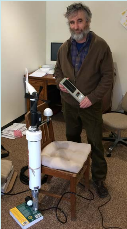
NEFSC oceanographer Jim Manning with a weather station and satellite transmitter that make up the shipboard weather stations being field tested now.
