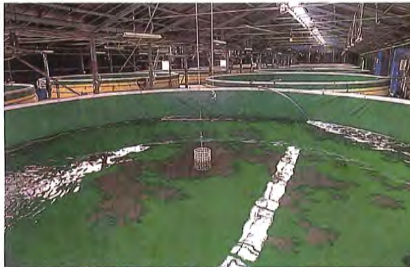
This is a bastard halibut culture facility in Asahi City, Chiba Prefecture, located about 10km inland from the coast. Seawater is supplied to the facility every day by means of a 30-ton tank lorry, and the water is circulated through a filtration system while in use. Because it is a closed life environment the water temperature is maintained in a range from 20 – 25°C. The facility is made up of 30 tanks, each 8m in diameter, and the production schedule is aimed at 60,000 adult fish per year. This highly unique culture operation is a joint venture between a pig raiser and a manufacturer of water purification equipment.
